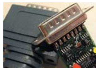
Figure 7. Overmold PCBA solution.
