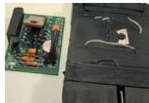
Figure 4. Direct premold, prior to overmold.
